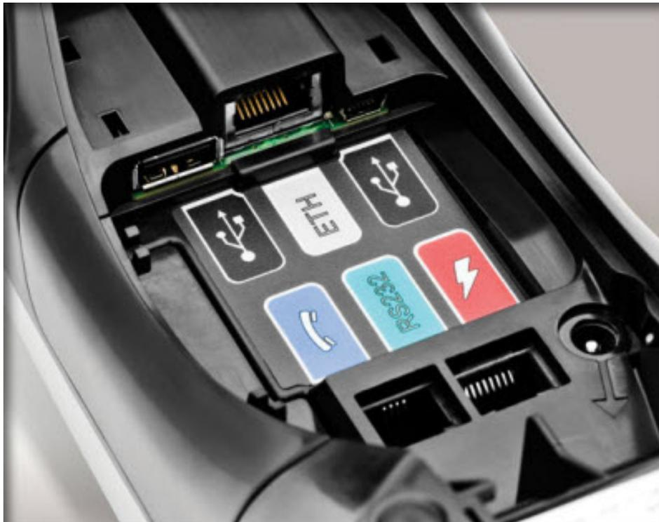
The pin pad cord comes connected in the RS-232 port.
