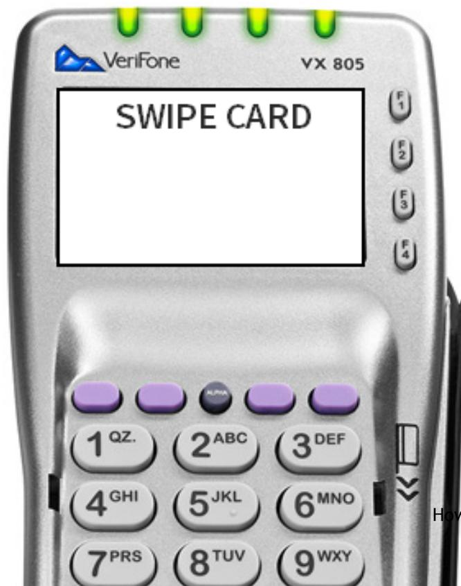
*Note: If the card will not swipe (the magnetic strip is worn or damaged), after 3 bad swipes, you will be prompted to manually enter the card number, expiration date, CV2 Code and card billing address Zip Code by using the key pad on the terminal.*
