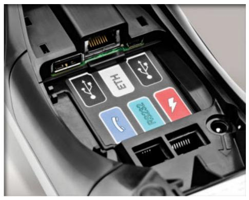
The pin pad cord comes connected in the RS-232 port.
